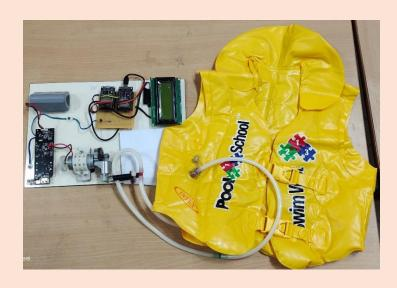
• This device integrates smart mobility aids—a smart shoe, walker, and air inflation tube—into a unified assistive system for real-time fall prevention and mobility enhancement. Utilizing IoT and AI, it enables remote monitoring and predictive care via ThingSpeak, supporting independence while allowing caregivers timely intervention.
