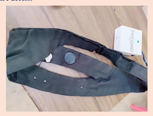
• The PREGAID Smart Belt revolutionizes maternal health monitoring with a wearable, low-radiation device that continuously tracks vital signs via IoT and shares data with healthcare providers through a mobile app. Compact and user-friendly, it supports remote monitoring and early interventions, making it invaluable for high-risk pregnancies, especially in underserved areas.
